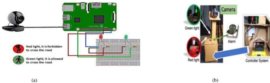
Figure 4. The implementation of the pelican crossing system for predicting the pedestrian age, (a) Schematic, (b) Our Prototype
